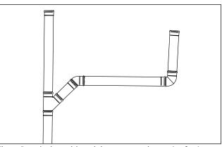
Fig. 5. Branch pipes with a minimum connection angle of 45° can be used when connecting ventilated side pipes.
