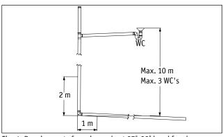
Fig. 1. Requirements for using a short 87°-88° bend for change from vertical to horizontal pipe run.
