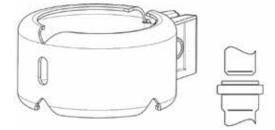
Appropriate fixing to the building can prevent the joints from sliding apart in most cases, but if it is difficult or impossible to fix the pipes to the building, joint clamps (type 847.xxx. xxx) can prevent the push-fit sockets and spigot ends from sliding apart if the system is overloaded or internal pressure is generated.
