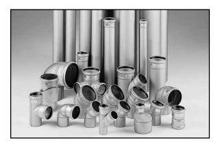
The BLÜCHER® EuroPipe drainage pipework system consists of pipes and fittings in stainless steel grades AISI 304 and 316L with socket and lip sealing ring. Available in 40, 50, 75, 82, 110, 125, 160, 200, 250 and 315 mm pipe diameter sizes and in standard lengths from 0,15 to 6 metres BLÜCHER® EuroPipe is a versatile, lightweight and easy-to-install pipework system.
