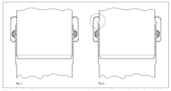
Joint clamps can be used in two ways: They can simply be tightened (see Fig. 1), or the spigot end can be provided with projections for the clamps to grip (see Fig. 2).
