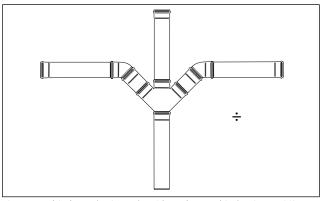
Fig. 7. Double branch pipes should not be used in horizontal lines.
