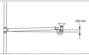
Fig. 1. The vertical distance between water surface in the water trap and bottom of the side pipe should be at least 100 mm.
