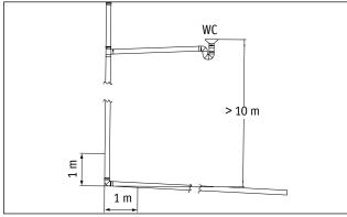
Fig. 6. No sanitary units should be connected closer than 1 m from the change of direction from vertical to horizontal pipes if a toilet is connected more than 10 m above the change in direction.
