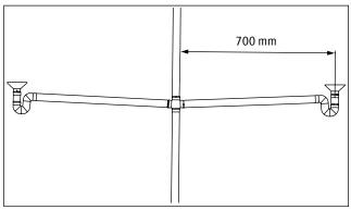
Fig. 4. When using double branch pipes with connecting angles larger than 45°, no sanitary units should be connected to the side pipes closer than 700 mm to the vertical pipe.
