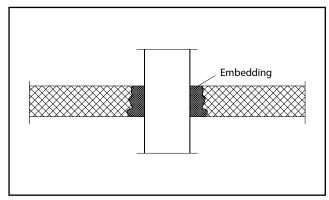
Fig. 1. Embedded non-combustible drainage pipe.
