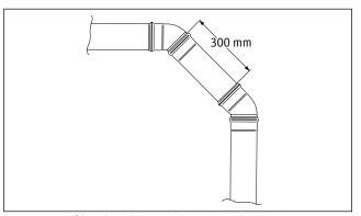
Fig. 4. Two 45° bends with a straight pipe section of at least 0.3 m between the bends should be used for 90° changes in direction.
