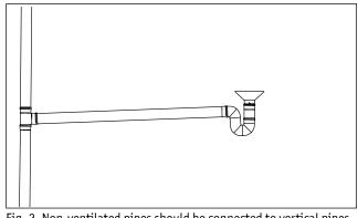
Fig. 2. Non-ventilated pipes should be connected to vertical pipes with 87°-88° branch pipes and the side pipe should have the smallest possible fall.
