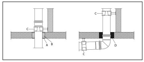
Fig. 3. Examples of fixing of non-combustible drainage pipes. A: Sealant. B: Mineral wool. C: Pipe bracket. D: Embedding.
