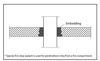
Fig. 2. Low-noise and fire-safe penetration of non-combustible drainage pipe.
