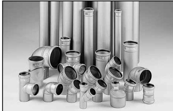
The BLÜCHER® EuroPipe drainage pipework system consists of pipes and fittings in stainless steel grades AISI 304 and 316L with socket and lip sealing ring. Available in 40, 50, 75, 82, 110, 125, 160, 200, 250 and 315 mm pipe diameter sizes and in standard lengths from 0,15 to 6 metres BLÜCHER® EuroPipe is a versatile, lightweight and easy-to-install pipework system.
