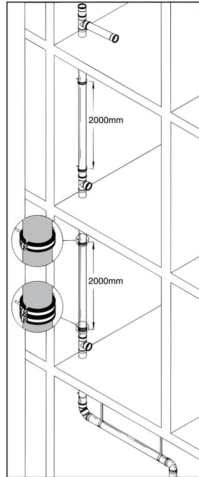
Test installation in accordance with EN 14366.
