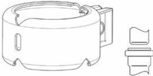
When installing the clamp joint please note that the two slices on the clamp should be at the socket end. Likewise, the one slice on the clamp should be located at the spigot end.
