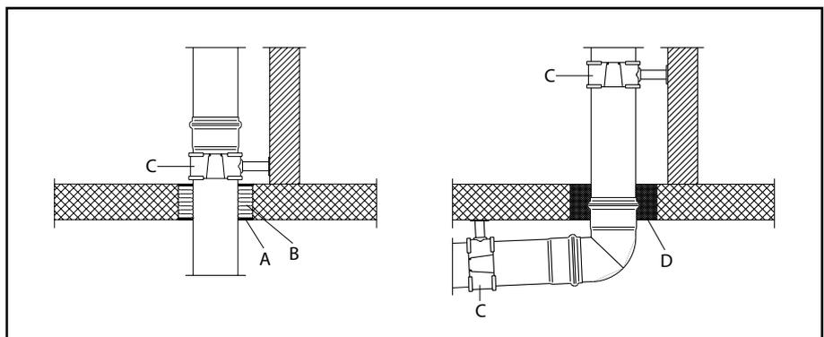
Fig. 3. Examples of fixing of non-combustible drainage pipes.
