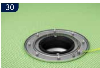
**(UK)** For a tight solution and to center the upper part over the lower part, place the sealing ring directly into the lower part. Fix the clamping ring with uniform torque. If an equipotential bond is required, connect the earth wire to the earthing screw at the upper edge of the membrane flange.
