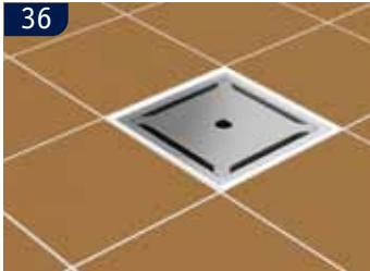
**UK** Insert water trap and filter basket. Install the grating, and the installation is complete.
