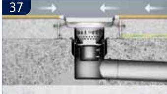
**UK** Sectional view showing the completed installation.
