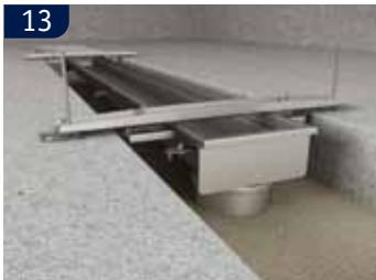
**UK** Channel mounting bracket type 670.000.000 (at least two per channel depending on channel weight and length) (to be ordered separately). Fix the channel to the mounting bracket at the correct height. Then fix the mounting bracket to the floor by means of screws to avoid the channel floating up during casting in the recess.
