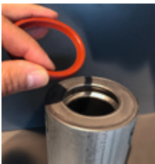
1) Remove sealing ring before welding
