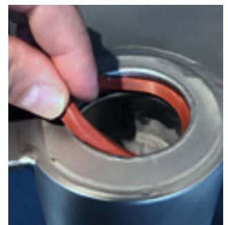
4) Insert sealing ring - be sure to turn it the right way
