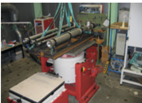
Test set up for the vibration test
