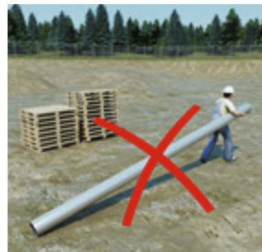
Pipes and fittings must not be dragged along the ground or other surfaces which could damage them.
