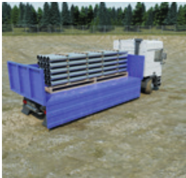
Pipes and fittings should be securely stored on pallets or packed to ensure that they do not rest on their sockets.
